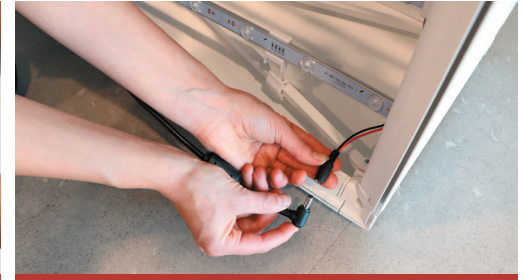
13. Connect the adapter to the LED curtain plug on the bottom side.
